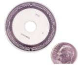
Unlike conventional code disks with a continuous repetition of opaque and transparent fields, the very small CoreTech<sup>™</sup> disk condenses absolute position information into one non-repeating circular barcode pattern. A second track with 1024 analog sine/cos cycles is used to enhance resolution and accuracy.
